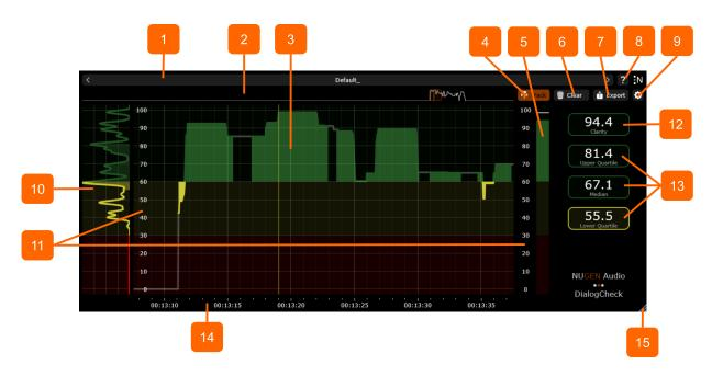
1 Preset Bar. Use the arrow buttons to step sequentially through the presets
