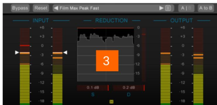
This scrolling history shows input level in grey, and the gain reduction applied in red. This visualisation can be useful to see how much gain is being applied over time, which can be difficult to assess using standard reduction metering. The effect of the look ahead and release controls can also be examined.
