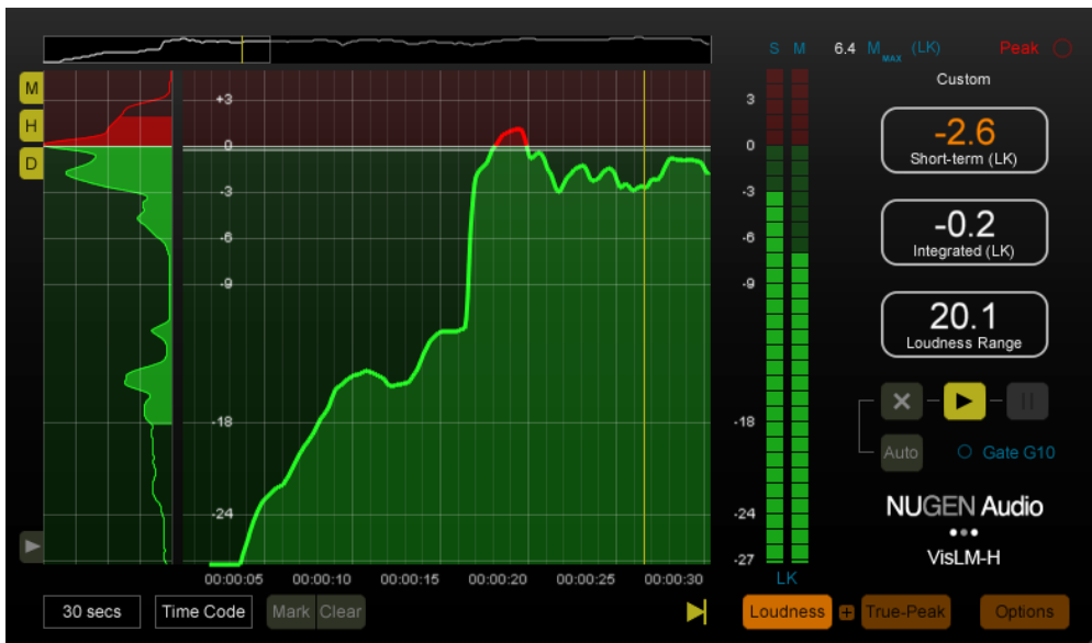
Fig 2. VisLM-H showing a 'green zone' Short-term Loudness range, with a no-go zone highlighted in red.
