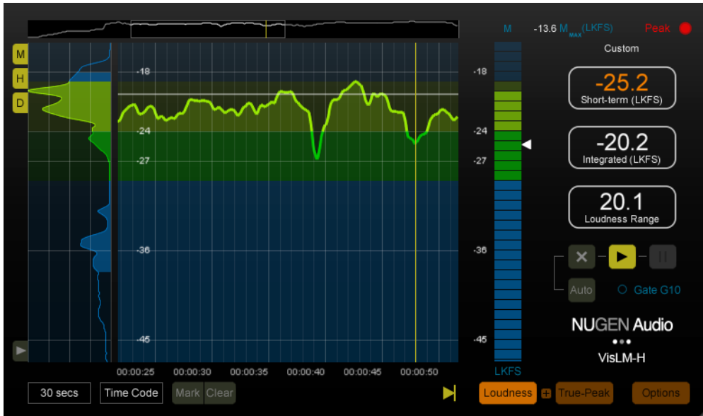
Fig 1. VisLM-H showing a preferred 'green zone' Short-term Loudness range, with a target loudness of -24 LKFS defined by a change in shading.
